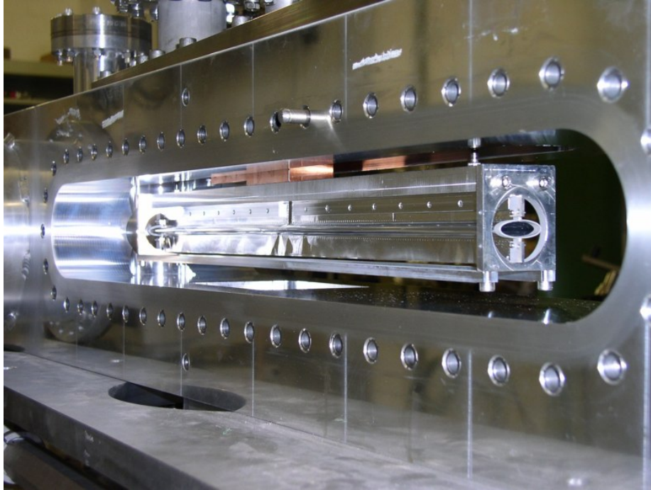
Figure 3-5: The OLYMPUS target cell, mounted within the aluminum scattering chamber (with the windows and wakefield suppressors removed) [124].
