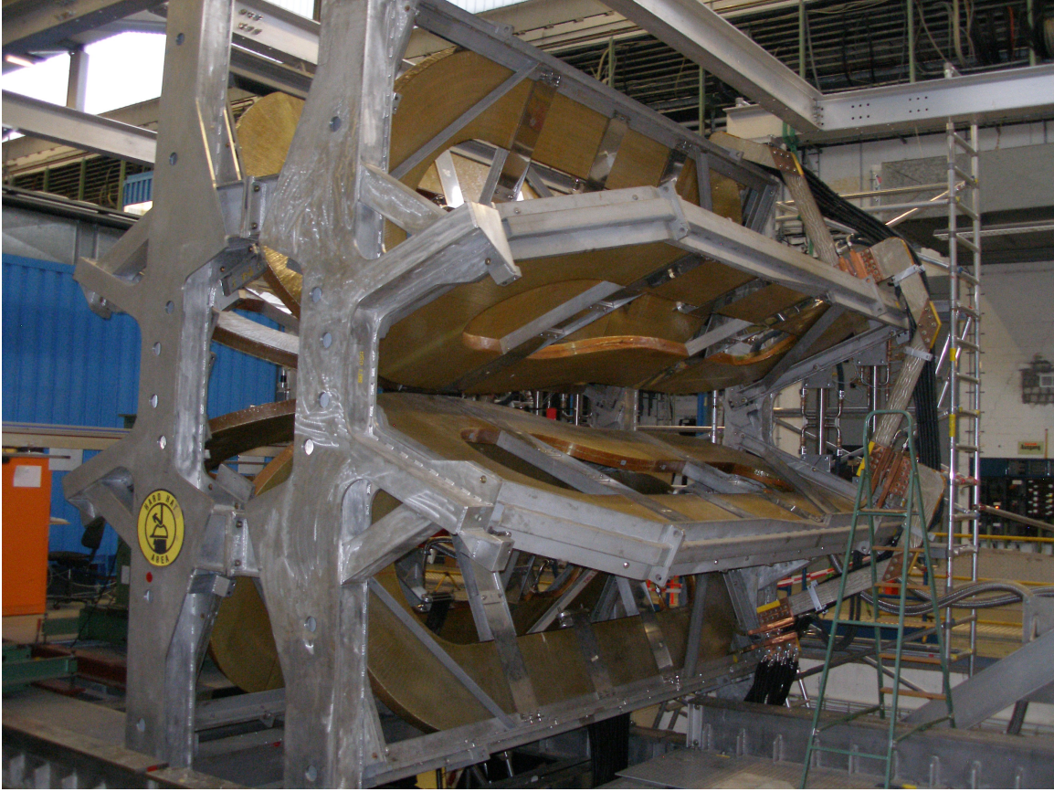
Figure 3-8: Photograph of the OLYMPUS toroid prior to installation in the DORIS beamline, showing the symmetric arrangement of the eight coils [38].
