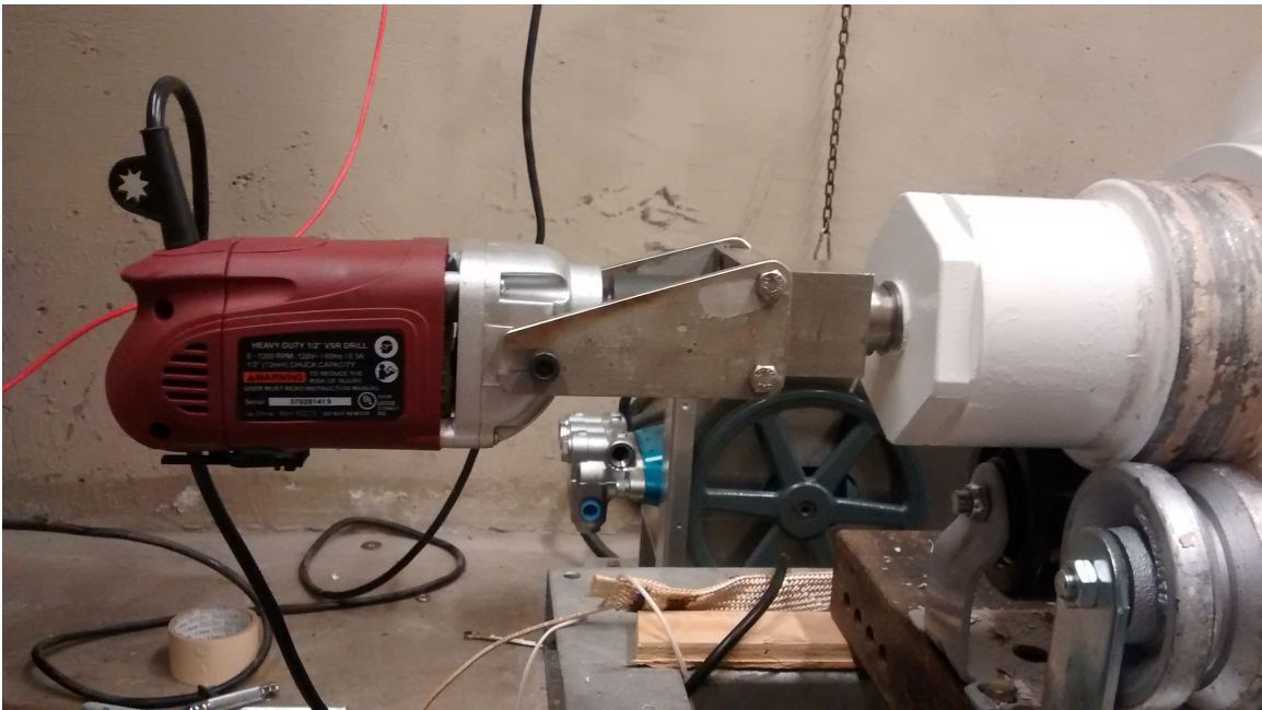
Figure 3-8: Mixer motor Installed in the tank bullplug
