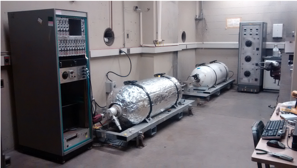
Figure 3-16: From left to right: electronics rack, charge tank, test section, dump tank, heater control
