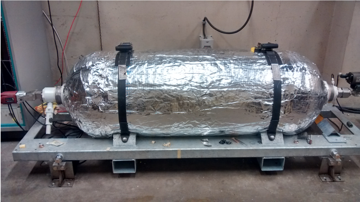
Figure 3-15: insulated charge tank
