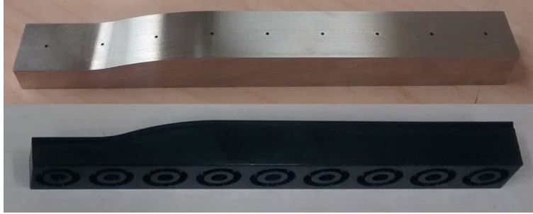
Figure 4-18: Comparison between original nozzle inserts and the second set of incorporating the o-ring groove and black anodization
