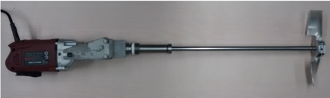
Figure 3-7: Mixer motor assembly outside the tank
