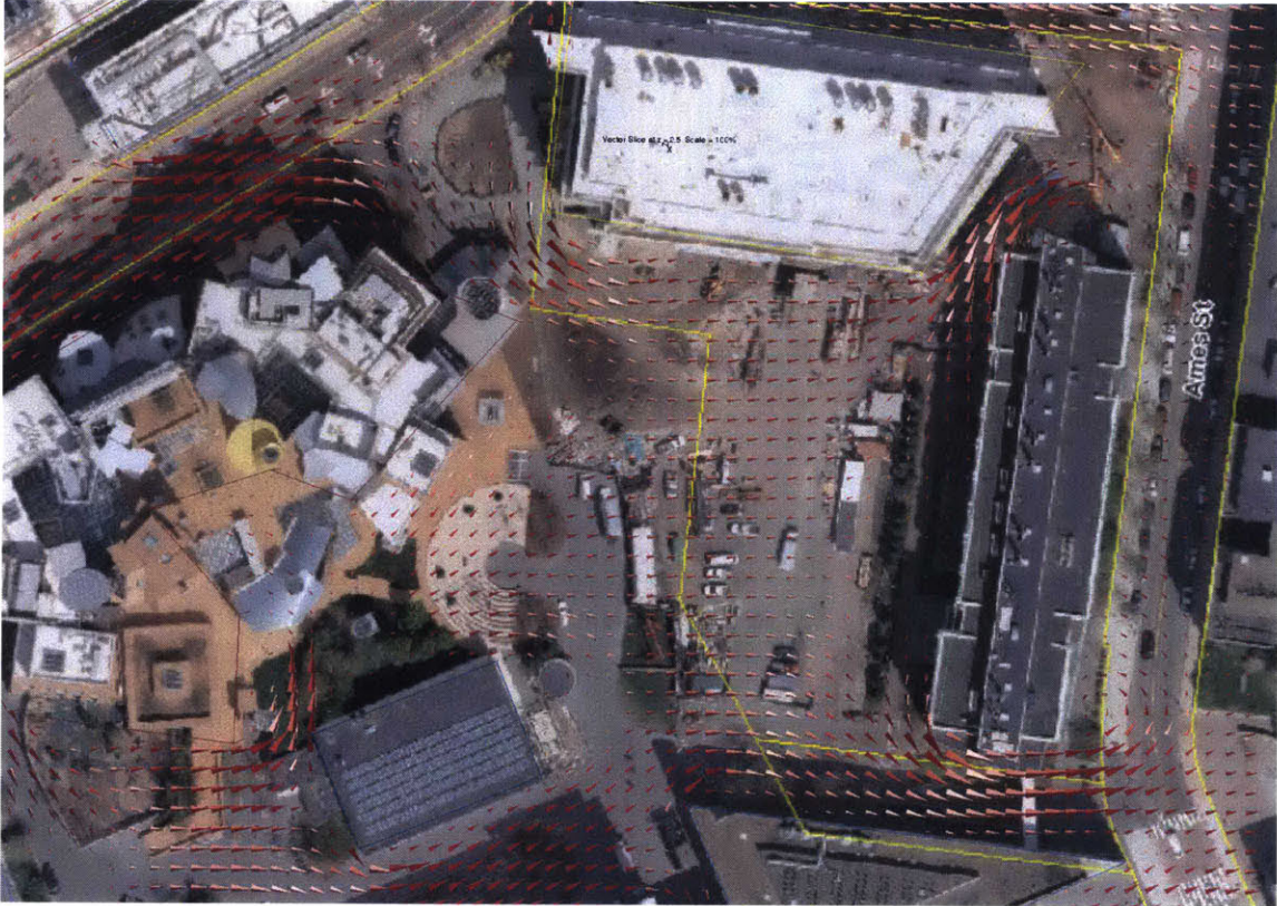
Figure 4-6: QUIC-CFD sample wind fields over a small region of MIT campus. The more traditional approach of QUIC-CFD eliminates the non-physical regions found in the QUIC-URB wind field for this environment.
