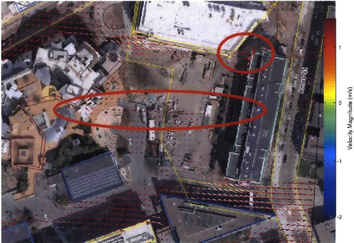
Figure 4-5: QUIC-URB sample wind fields over a small region of MIT campus. The approximations taken in the solver introduce clearly non-physical regions within the wind field that are circled in red.
