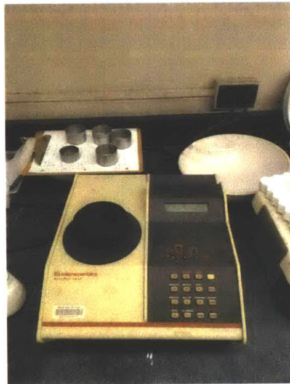
Figure 3.16: AccuPyc1330 gas pycnometer used for oven-dried solid density measurements
