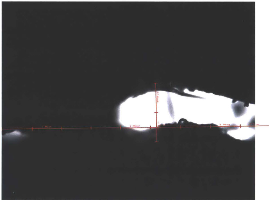
Figure 3-2) 1000 micron hole in waxed cotton with measurement line. The hole is about 900 microns long and about 200 microns wide.
