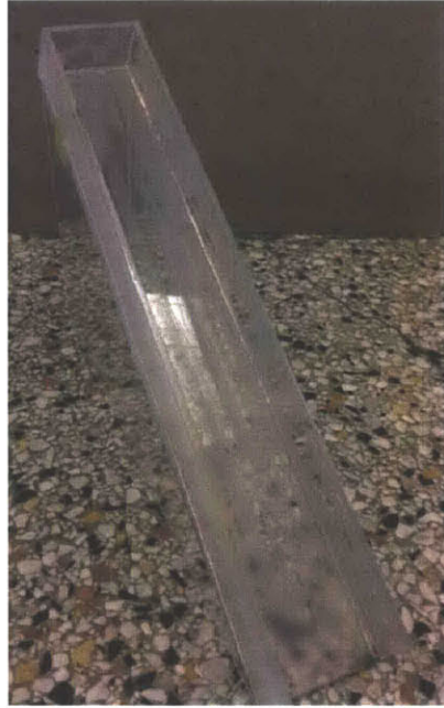
Figure 3-7) The acrylic channel used to measure the viscosity of the mixtures of Elmer's glue and water.
