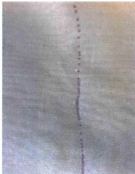
Figure 3-8) One of the tests done with the Elmer's glue mixture. Where the holes are close together, the adhesive forms a line instead of individual beads.
