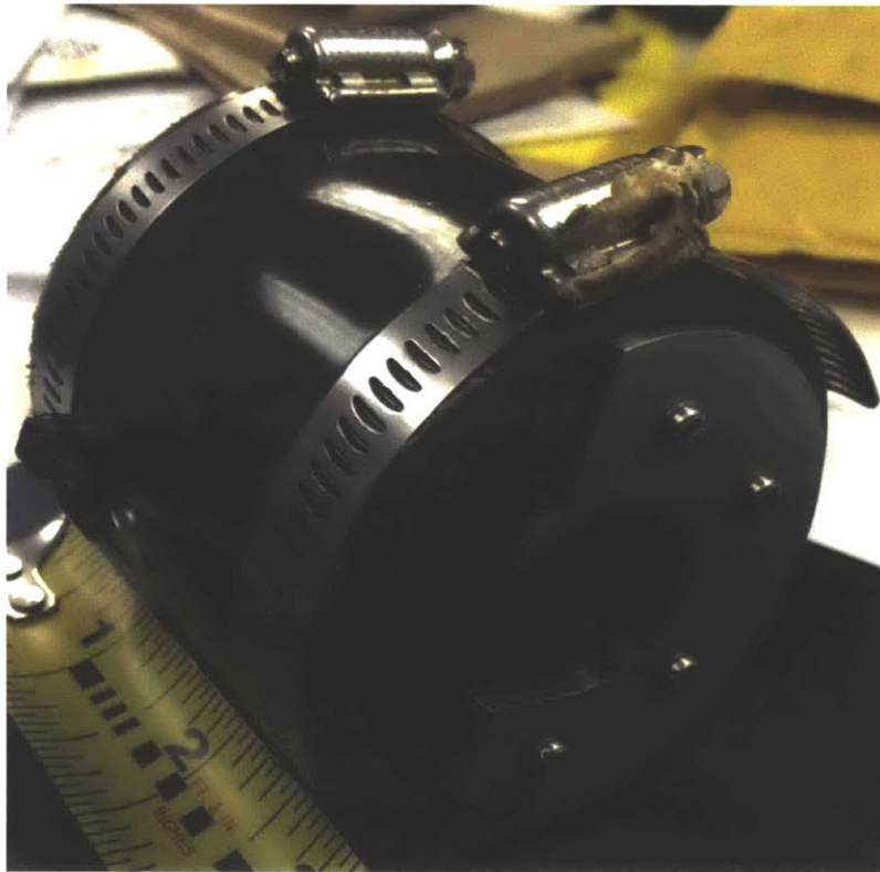
Figure 9: Commercially available corrosion cell for rotating beam fatigue tester
