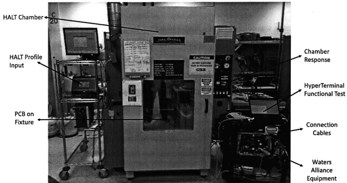
Figure 33 – Vibration step stress experimental setup
