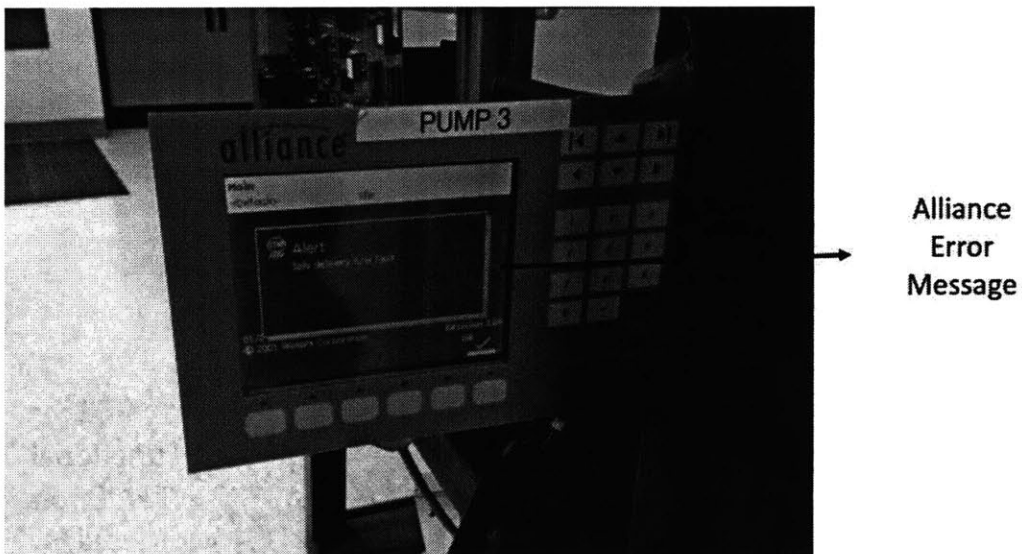
Figure 35 – Error message observed during vibrational step stress
