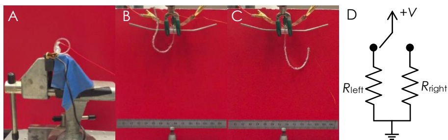
Figure 2 – (A) The nylon curled over two times which results in radius of curvature around 0.56 \text{ mm}^{-1} . (B) and (C) show radius of curvature around 0.23 \text{ mm}^{-1} for a reversible actuation.
