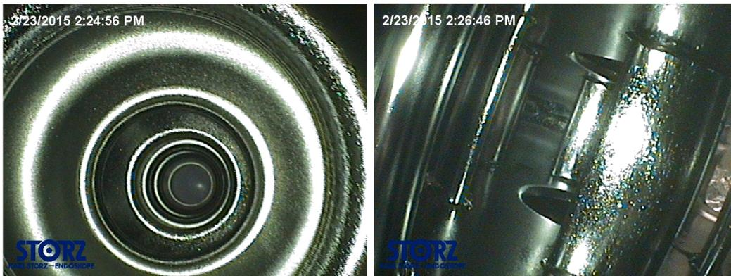
Figure 6-5: Photographs of the inside of the cavity, taken during the inspection. No visible defects were found.
