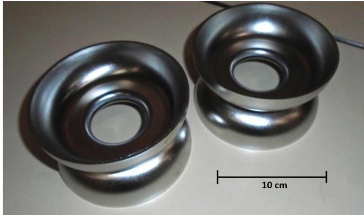
Figure 4-2: Two “dumbbells” used on the opposite sides of the five-cell cavity. Each dumbbells formed by two halves of the elliptical cells welded together at the irises.
