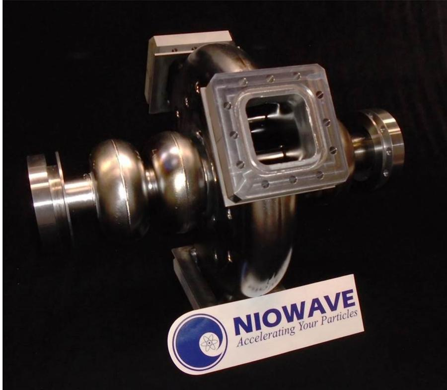
Figure 1-11: The fabricated niobium 5-cell accelerating cavity with a coupler PBG cell in the middle. The cavity resonates at the RF frequency of 2.1 GHz.
