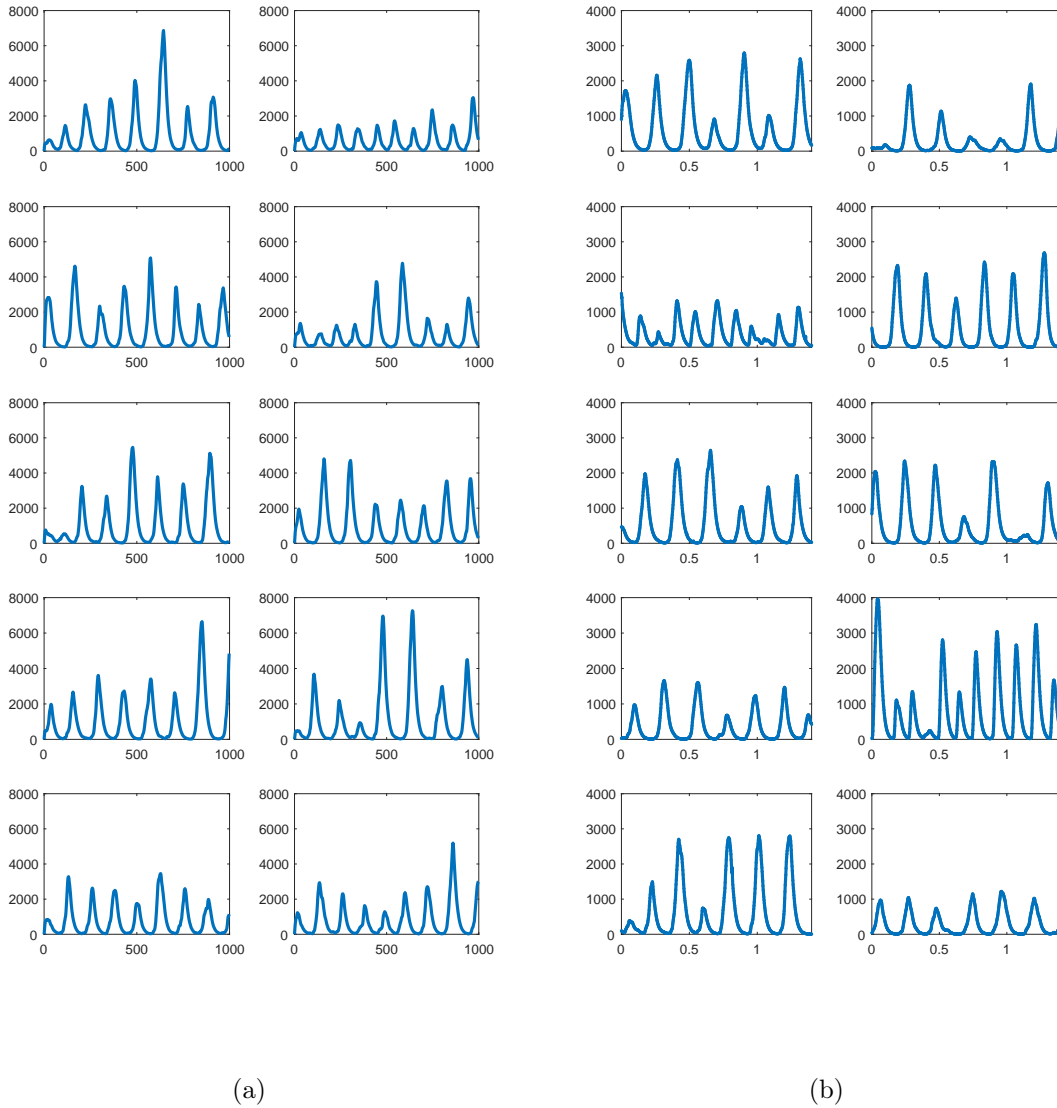
Figure 4-5: The waveforms for the levels of LacI molecules, obtained from stochastic simulations of the repressilator network (see Section 2.4.1), using (a) software (10 runs in series) and (b) the cytomorphic board (1 run in parallel). Units – (a) x axis: minute, y axis: number of molecules, (b) x axis: second, y axis: ADC output (1 ADC output \approx 2.5 molecule. Variations may exist among chips.)
