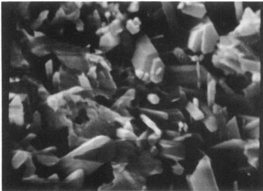
.A.2 Surface of A.1 at Higher Magnification. Crystals are Mixture of Calcium Sulfate and Calcium Carbonate.
