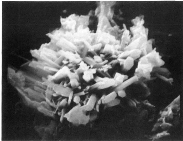
.A. A Radiating Group of Large to Small Calcium Carbonate Crystals. Some sulfur is also evident from EDXRA showing presence of some \text{CaSO}_4 type structure.
