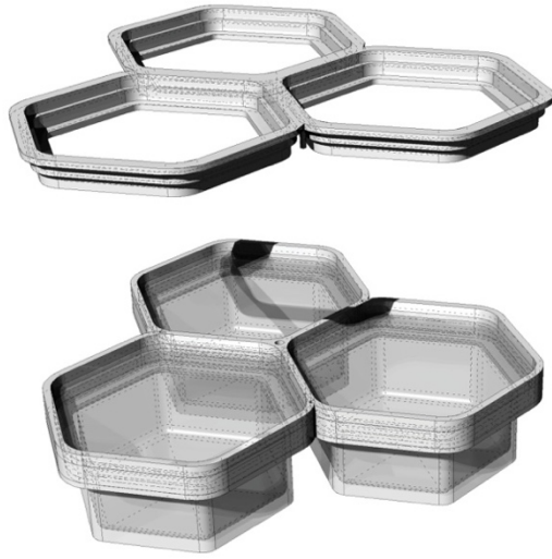
Figure 23: Growth vessels can be easily attached and detached to and from the system's frame
