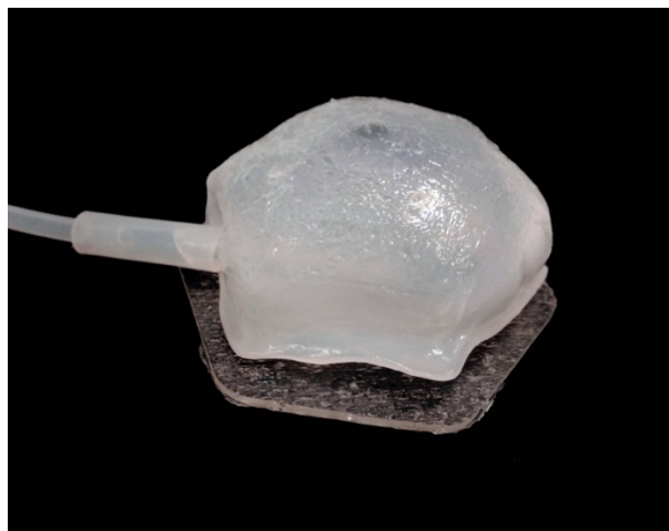
Figure 28: The BC-PVA composite after pneumatic actuation. Hydrogel state.
