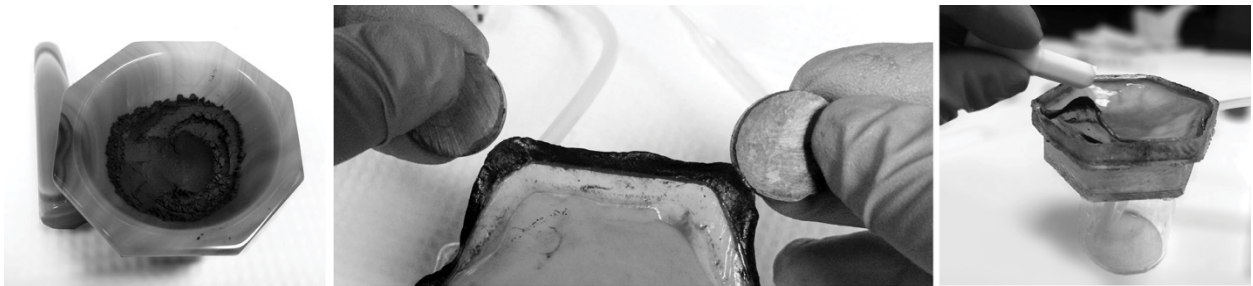
Figure 32: (left) Fe_3O_4 (Magnetite) particles. (middle and right) BC-Magnetite composites display magnetic features.
