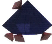
Figure 5-18: Initial contacts and linearized friction cones.
