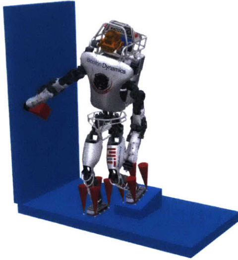
Figure 3-1: Atlas with multiple non-coplanar contacts.
