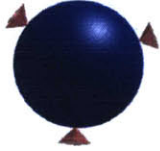
Figure 5-15: Optimized contacts and linearized friction cones.
