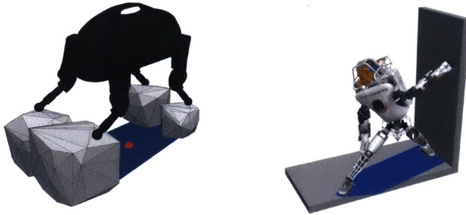
(a) Static Posture for Little Dog on step- (b) Static Posture for Atlas with foot and ping stones. The blue region is the sup- left hand contact. The robot stretches its port region for Center of Mass projection legs and arms to maximize the support (red dot). region (blue).
