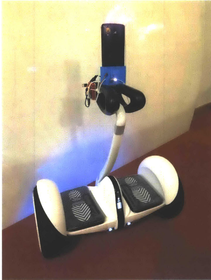
Figure 6-14: Smartphone LDS mounted on a self-balancing scooter.
