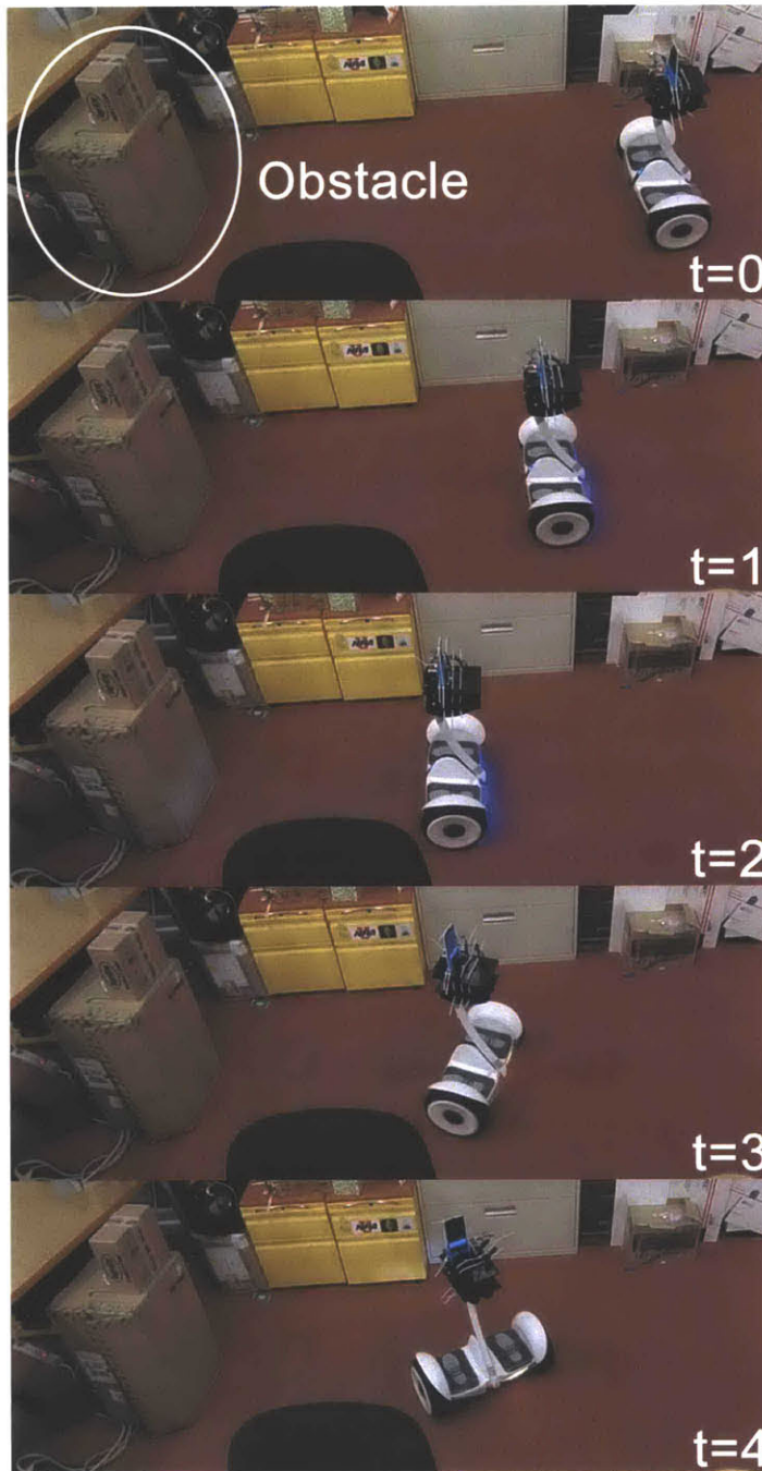
Figure 6-16: Video frames showing robot avoiding an obstacle.
