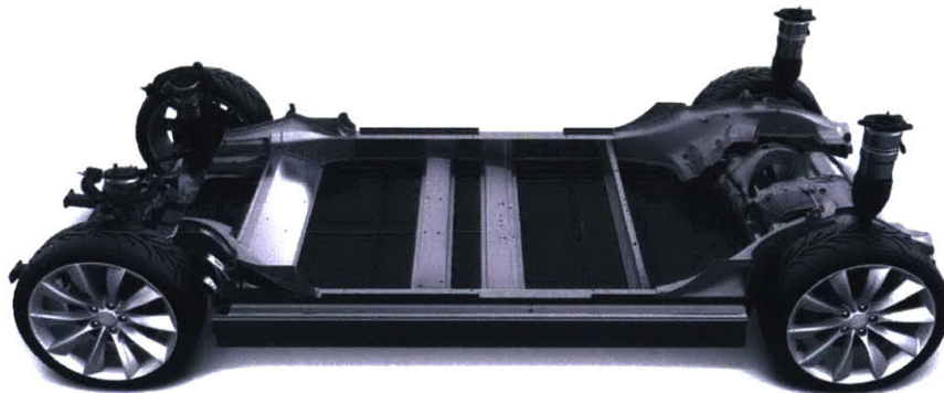
Figure 35: Tesla Model S battery pack underneath chassis sub-system components
