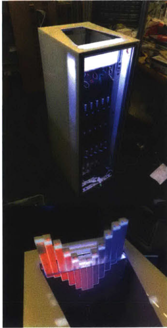
Figure 44 The first prototype of inForce using force sensors within the pins to render force feedback on a 12x1 pin array
