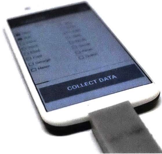
Figure 4.12. The mother node enables a smartphone to communicate to all sensors in the classroom.
