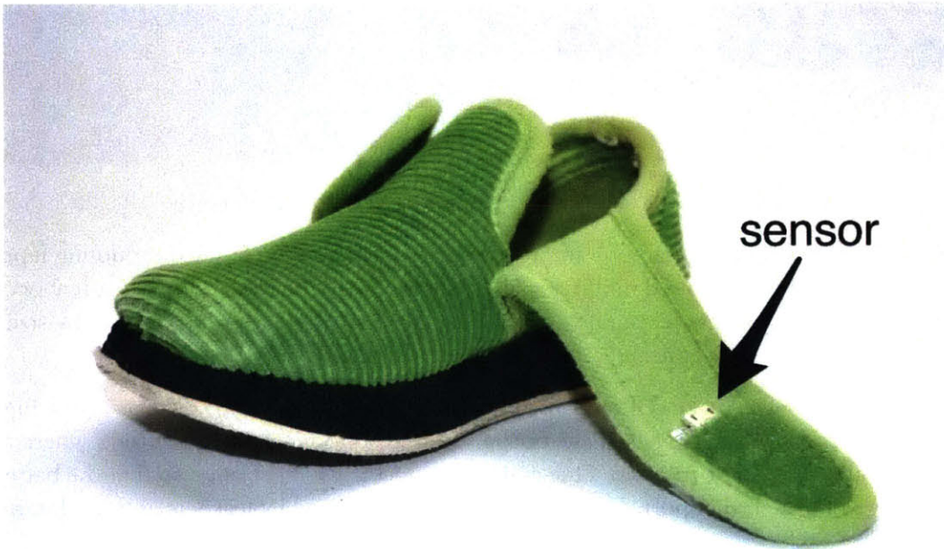
Figure 4.1 Modified shoe that can house a 2cm x 2.5cm PCB in a minimally invasive fashion.
