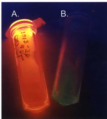
Figure 2-6: A photograph of two NB-Monodentate-coated CdSe-CdS samples under UV-illumination displaying different levels of stability in water; each of them represents a particular CdS shell synthesis method. (A) Stable CdSe-CdS QDs derived from a method described by Chen et al. [4] and using OA as the main surface ligand. (B) Aggregated CdSe-CdS QDs derived from a method described by Liu et al. [55] and using n -hexylphosphonic acid as the main surface ligand.
