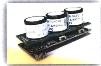
Figure 10: Second revision, Atmel based learnAir main board mated with the AlphaSense sensor frontend
