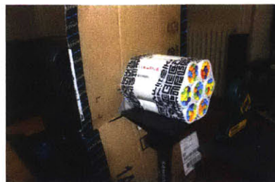
Figure 19: A picture of a simple laminar flow test setup for rough wind directivity characterization
