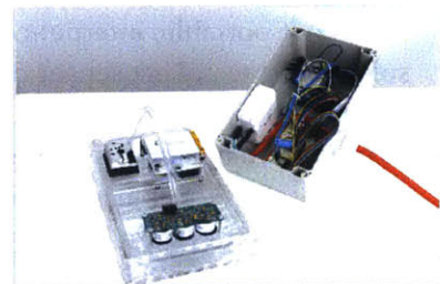
Figure 3: LearnAir Sensor installed at MassDEP site, opened
