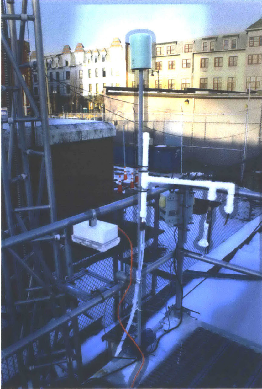
Figure 8: LearnAir Sensor (box on left) installation next to MassDEP inlet (top of pole on right)
