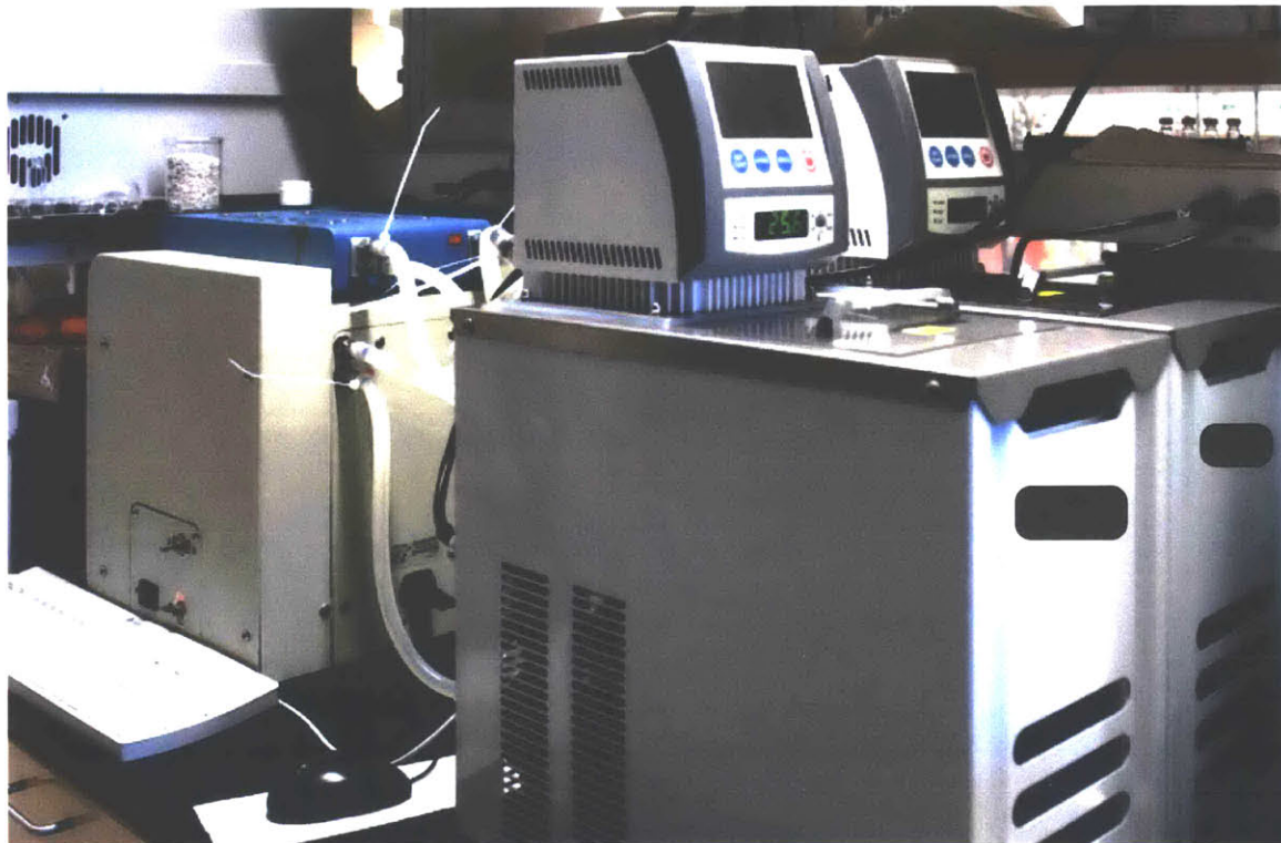
Figure 1-8 Omnical Calorimeter with circulating cooling/heating baths. Note: The “brand names” of the circulating coolers have been edited out of the picture
