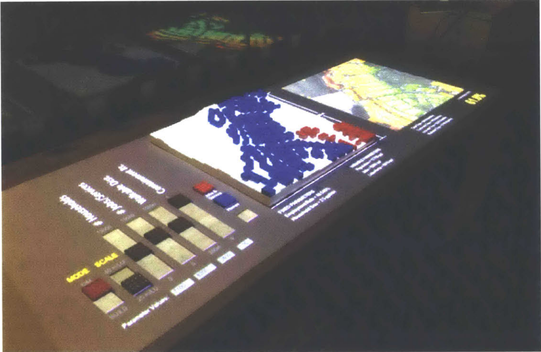
Figure 11: CityScope MarkII Scout Table, using static projection mapping onto a canvas for land use planning, allowing rapid prototyping with real-time evaluation (Larson, Reinhart, Alfaris, & Al-Wabil, 2014).
