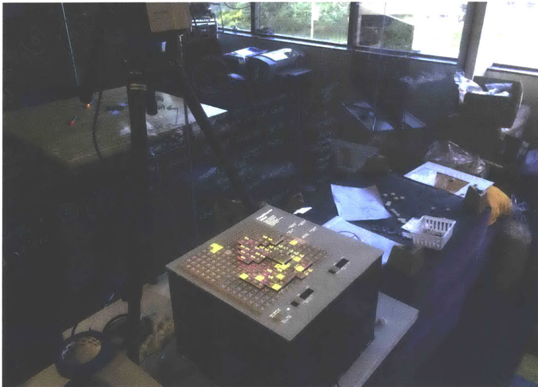
Figure 21: Overview of the CityMatrix— an urban vitality computational evaluation tool. There are three main physical components to the platform: the Lego table, overhead projection, and camera (for reading Lego tags)
