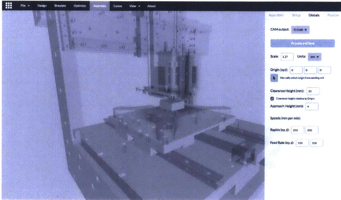
Figure 3-8: Interface for defining global assembly variables such as lattice pitch, machine origin, clearances, and feed rates.
