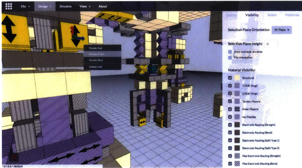
Figure 6-1: A schematic diagram of a robotic “pick and place” in AMOEBA. Cell rotation GUI allows anisotropic cells to be oriented in any direction.
