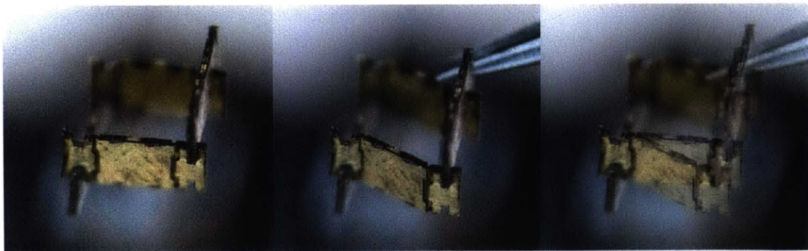
Figure 7-3: Large angular deflection of bending flexures in a small assembly of functional parts. Image Credit: Will Langford 2016
