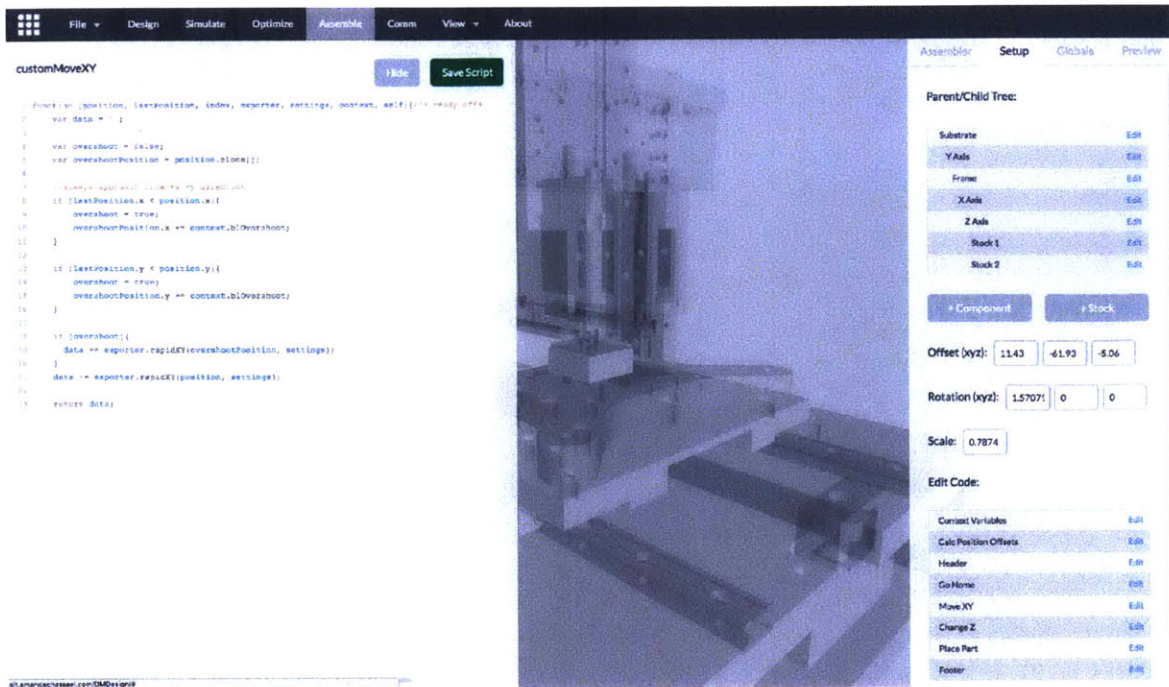
Figure 3-11: Scripting interface for custom machine configuration. This screenshot shows a user-defined function that calculates XY traversals with added backlash compensation specific to the “Stapler” assembler. Other user-defined functions are listed in the bottom right, including: context variables, header, place part, footer, and others.
