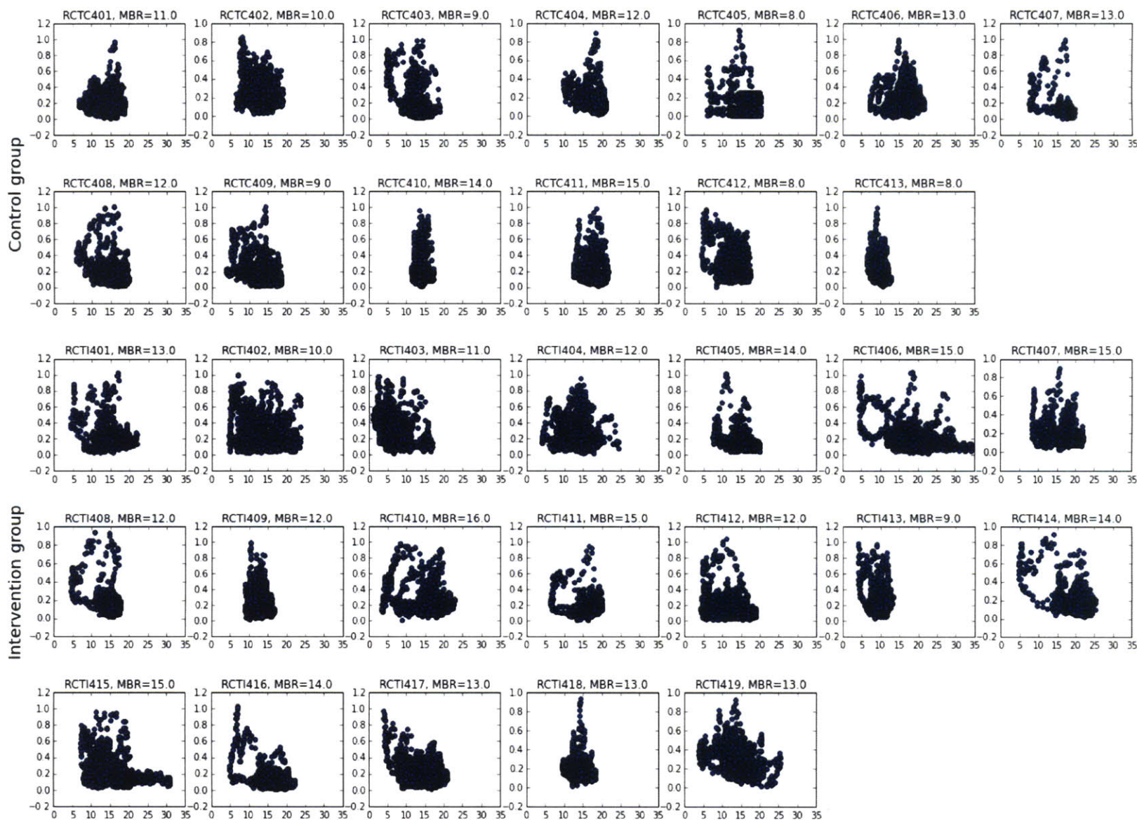
Figure A-5: Main - Normalized amplitude versus breathing rate for each user. The individual MBRs are written on top of the plots. The intervention users have points under lower rate and higher amplitude that stand out from majority of the points. However, for the control users, higher amplitude points have higher relative rate.
