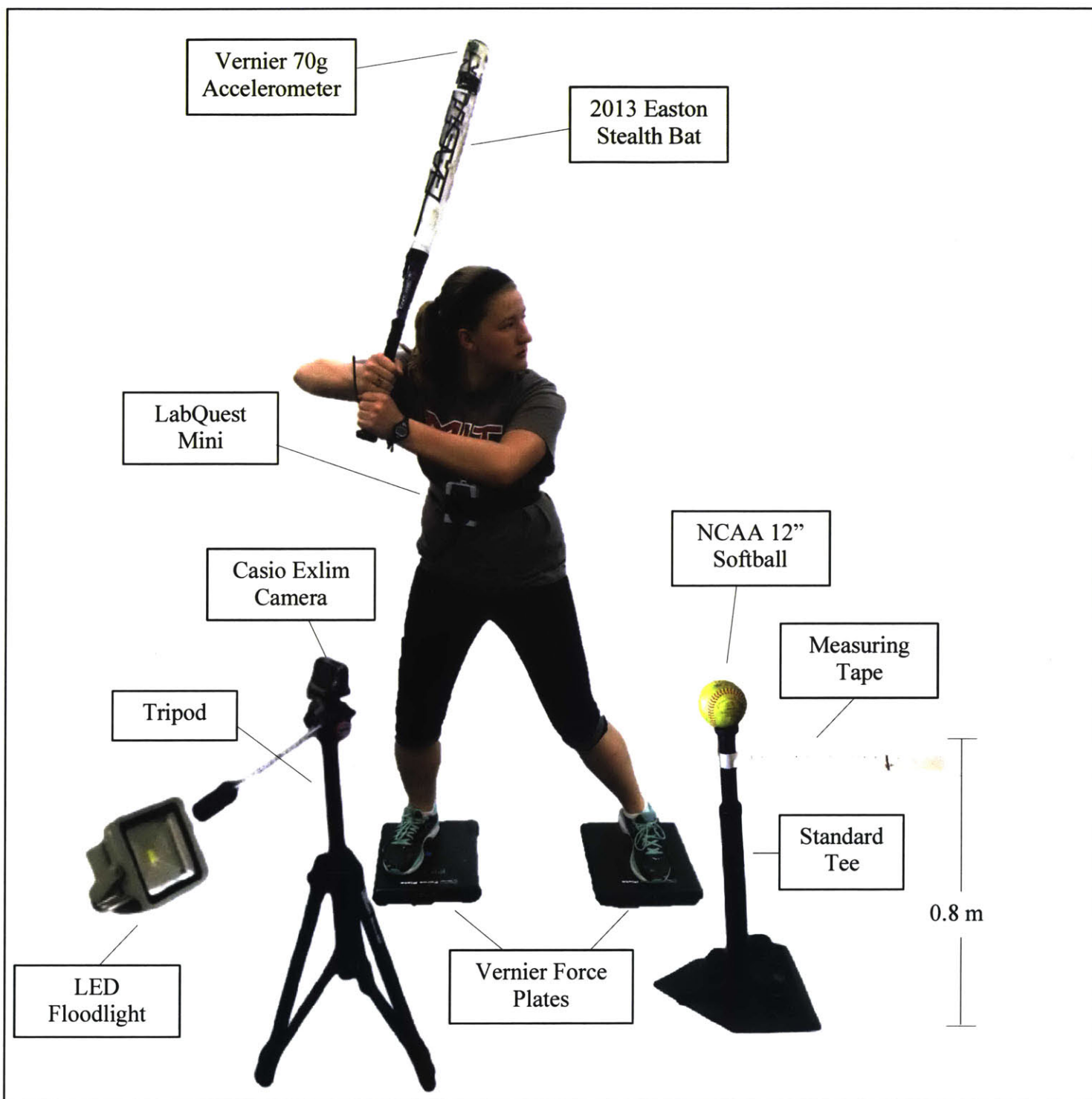
Figure 8: This diagram displays the setup used to determine the weight shift, the bat velocity and the ball velocity. As shown, the batter is hitting a ball off of a tee, while being filmed by a Casio EXLIM high-speed camera at 1,000 frames/second. The LED floodlight provides lighting to obtain better video quality. Simultaneously, the player stands on two force plates, and the force applied to each plate during the swing is recorded through the LabQuest Mini and LoggerPro. A Vernier 70g accelerometer is attached to the end of the 2013 Easton Stealth bat to record the centripetal acceleration.
