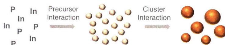
Figure 2-8: A two-stage growth model of InP QDs
