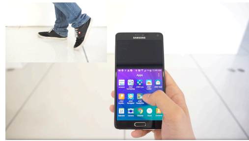
Figure 4. The user is moving his foot backwards to make the screen of the phone move accordingly.
