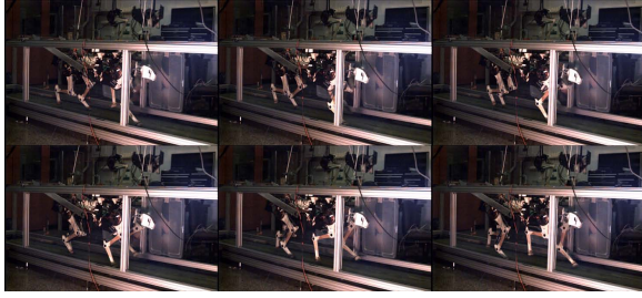
Fig. 14: High-speed video captured at 500 fps depicting 150ms of the MIT Cheetah running at 6 m/s.
