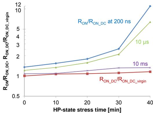
**Fig. 3** Dynamic  $R_{ON}$  ( $R_{ON}/R_{ON\_DC}$ ) of Fig. 2 at different times (200 ns, 10  $\mu$ s, and 10 ms) and  $R_{ON\_DC}/R_{ON\_DC\_virgin}$  ( $R_{ON\_DC}$  value in the virgin device) as a function of HP-state stress time in a semilog scale. Dynamic  $R_{ON}$  mostly increases in a time range from 200 ns up to a few ms.  $R_{ON\_DC}/R_{ON\_DC\_virgin}$  shows small increase up to 16% in comparison to dynamic  $R_{ON}$  suggesting minor permanent (non-transient) degradation.
