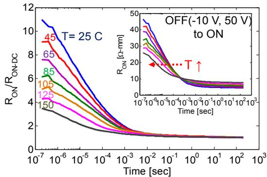
**Fig. 5**  $R_{ON}/R_{ON\_DC}$  transients at different temperatures between 25 C and 150 C for  $V_{GSQ} = -10$  V and  $V_{DSQ} = 50$  V after 40 min HP stress. The inset shows the absolute value of the  $R_{ON}$  transient. As the temperature goes up, the dominant transients are substantially accelerated. This suggests that the transients are due to generated traps.
