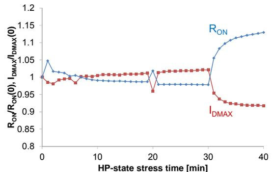
**Fig. 1** Time evolution of  $R_{ON}$  and  $I_{D_{MAX}}$  (normalized to their initial values) during a constant HP-state stress in GaN HEMTs. The stress conditions are  $V_{GS} = 2$  V, and  $V_{DS} = 20$  V. Up to about 30 min of stress, the device characteristics show minor changes. Beyond 30 min, prominent degradation in both  $R_{ON}$  and  $I_{D_{MAX}}$  is observed.
