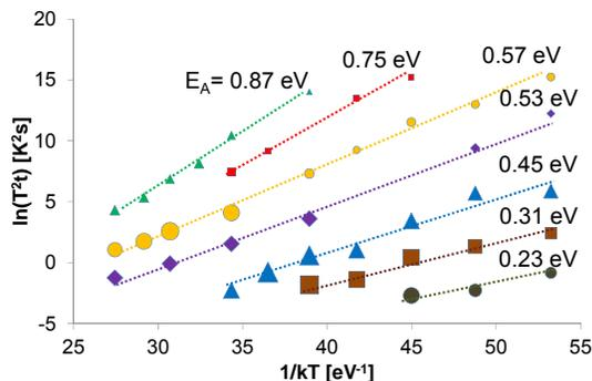
**Fig. 6** Arrhenius plot of time constant spectra extracted from **Fig. 5**. The size of the symbols is proportional to the height of the time constant peaks. The dominant trap energy levels are located at 0.31, 0.45, 0.53 and 0.57 eV below the conduction band edge of the AlGaIn barrier. These are the traps that are responsible for the dramatic increase in dynamic  $R_{ON}$  that is observed in a short time scale.
