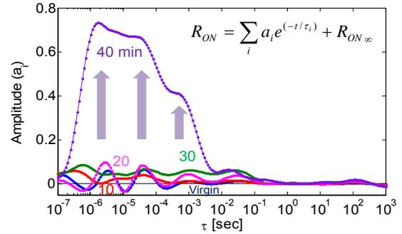
**Fig. 4** Time-constant spectra for  $R_{ON}$  transients of Fig. 2. A sum of exponential terms with time constant ranging from  $10^{-7}$ s to  $10^3$ s is used to fit the measurement data. The appropriate equation for fitting is indicated in the inset. After 40 min of stress, there is a prominent increase of the magnitude of transients with short time constants.
