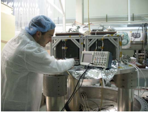
Fig. 20. Custom electric cables routed along the suspension wires.
