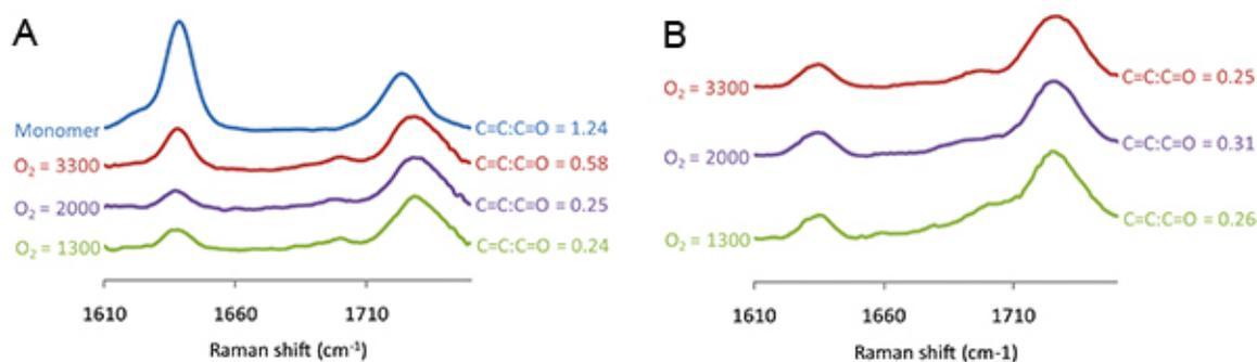
**Figure 7.** The Raman spectra measured for polymer spots of 4-tert-butylcyclohexyl acrylate printed at varied O<sub>2</sub> levels, indicated to the left of each spectrum, (A) before and (B) after vacuum extraction. The ratio of the Raman intensity for the C=C Raman shift at  $1640\text{ cm}^{-1}$  and the C=O Raman shift at  $1720\text{ cm}^{-1}$  is shown to the right of each spectrum.
