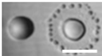
**Figure 8.** A light microscopy image of two polymer spots. The spot on the left shows a well formed spot, whilst the spot on the right is an example of a spot containing a very unevenly distribution of monomer. The scale bar is  $500\text{ }\mu\text{m}$ .
