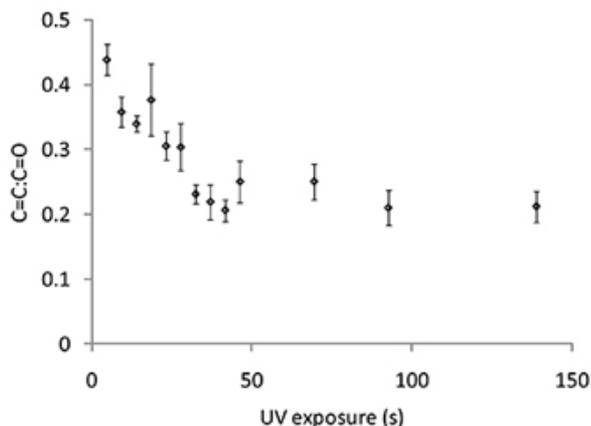
**Figure 6.** The ratio of the Raman intensity for the C=C Raman shift at  $1640\text{ cm}^{-1}$  and the C=O Raman shift at  $1720\text{ cm}^{-1}$  from polymer spots of 4-tert-butylcyclohexyl acrylate with varied UV exposure. The error bars equal one standard deviation ( $n = 3$ ).
