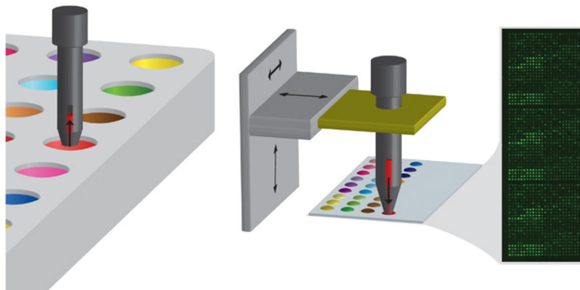
**Figure 2.** Schematic of the methodology of pin printing involving initially loading the pin with monomer in a source plate and then depositing the monomer onto a substrate by making contact. The pin is controlled by an X-Y-Z robotic arm. The inset shows a typical image of the autofluorescence from an array after production.
