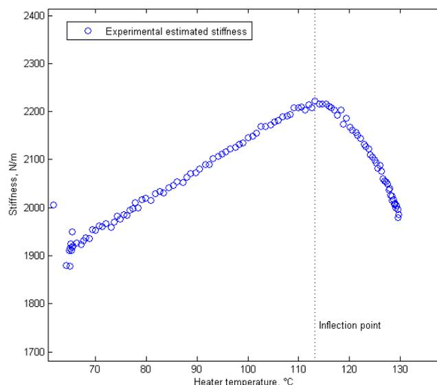
**FIGURE 7. EFFECTIVE STIFFNESS VERSUS TEMPERATURE MEASUREMENT, IN WHICH A CLEAR INFLECTION POINT MARKS A STEEP DROP IN STIFFNESS.**
