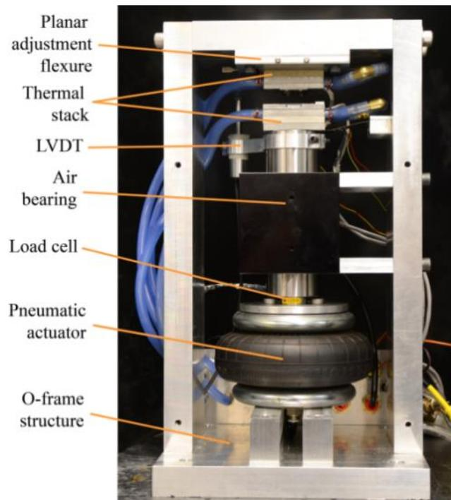
**FIGURE 1. EXPERIMENTAL EQUIPMENT WITH KEY FEATURES LABELED.**
