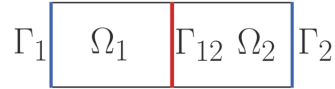
FIG. 2.1. Illustration of the decomposition of \Omega in \Omega_1 and \Omega_2 and the position of the ports \Gamma_1, \Gamma_{12}, \Gamma_2 within \Omega in a simplified two-dimensional setting.
