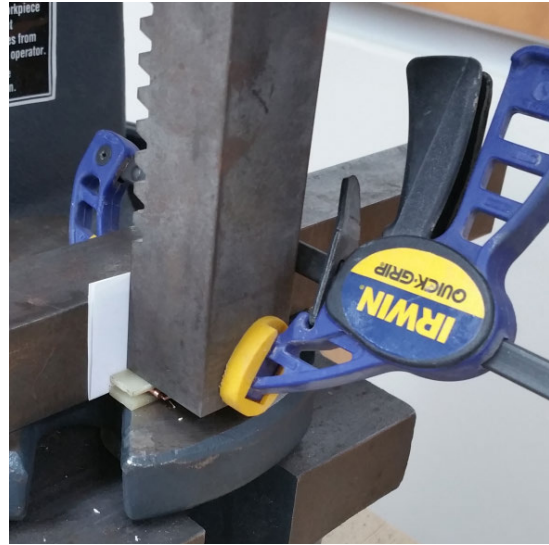
(b) Epoxy pairs of electrodes between the two support pieces of FR4 with 832HT-375 high temperature epoxy.
