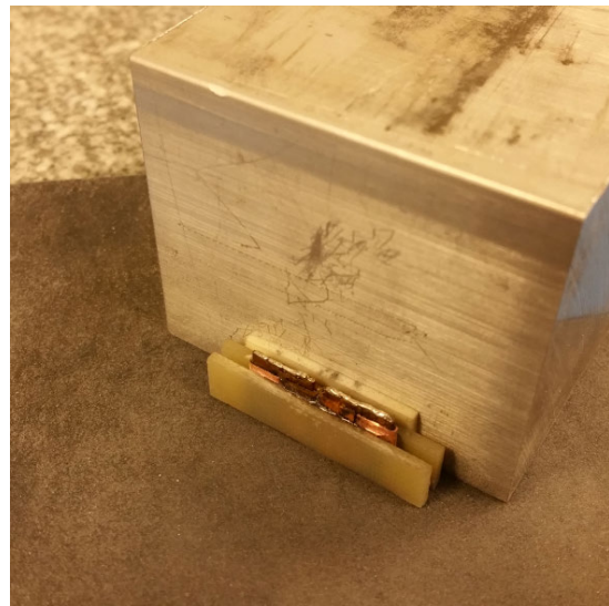
(d) Lap with increasing grit sandpaper and finally 2000 grit paste.
