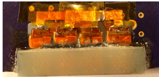
(f) Bottom view showing short-wavelength sense electrodes electrical connection to the drive electronics.
