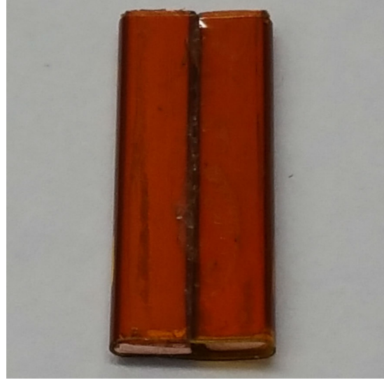
(b) Insulate with 0.064 mm (2.5 mil) Kaptan tape.
