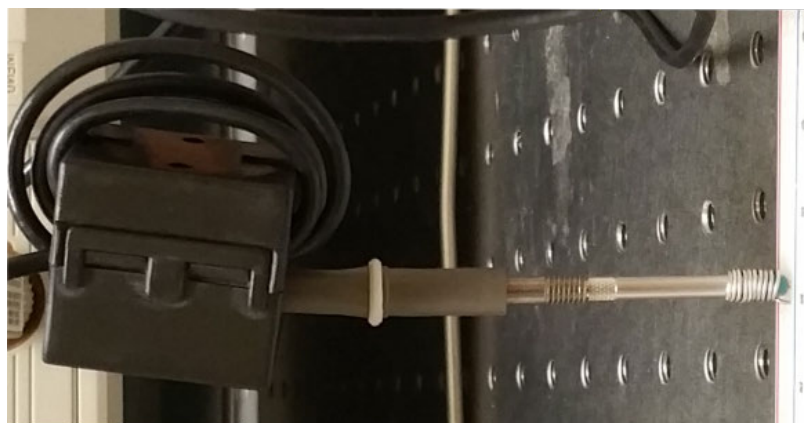
Figure C-2: Wrapping an oscilloscope probe around a ferrite core can further reduce outside noise picked up.
