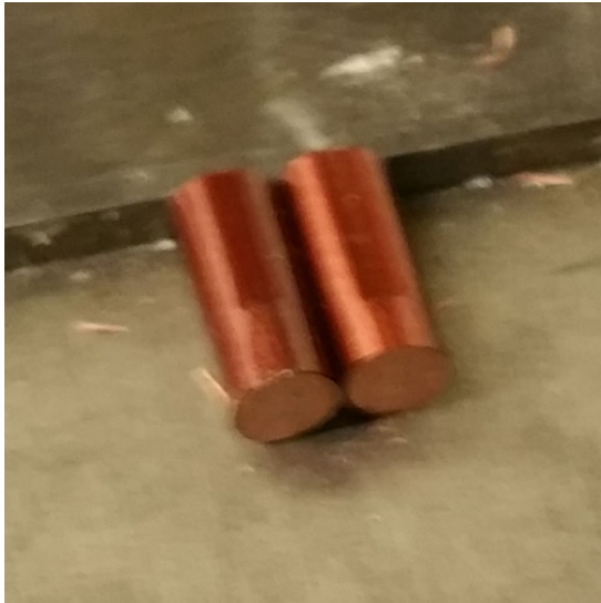
(a) Cut two strips of AWG 9 copper wire to make the sense electrodes.
