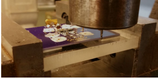
(a) Fixture drive electronic PCB in mill with double-sided tape.
