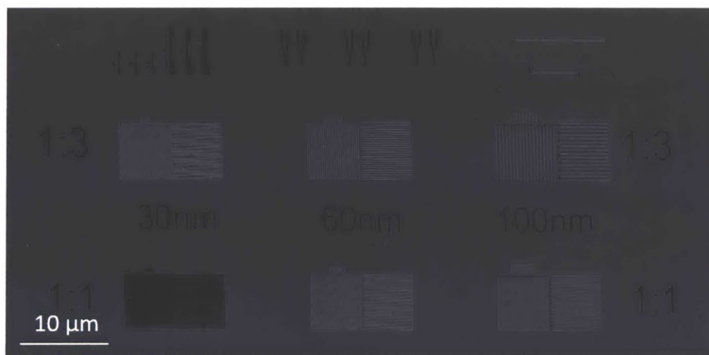
Figure 3-8: SEM of a unit cell of the standard dose matrix. The original pattern was designed by Adam McCaughan.
