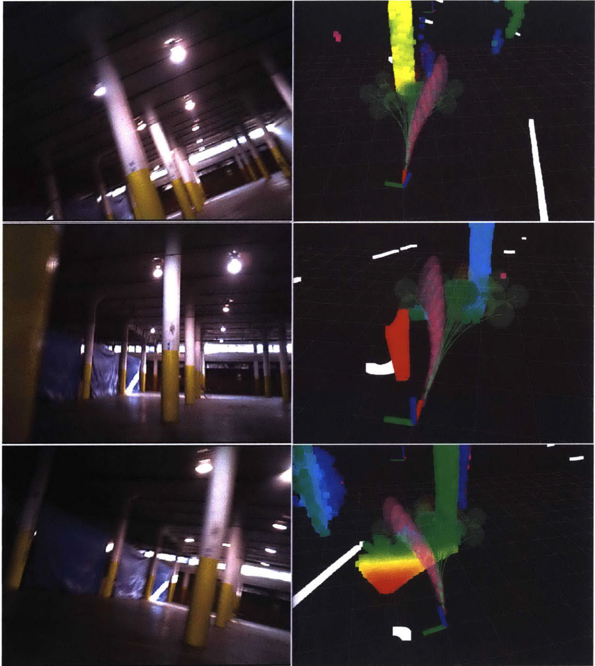
Figure 3-4: Outbound flight at 5 m/s. The vehicle approaches the second pillar at speed (top), then begins to roll left as soon as the previous pillar is passed (middle), taking this turn with a roll angle of approximately 25 deg (bottom).
