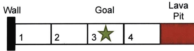
Figure 1-2: Toy example, inspired by Kaelbling et al. [7], of how a separation principle does not generally apply to POMDPs. In this example, the actions available are WEST and EAST . Entering the lava pit is irrecoverable, whereas attempting to enter the wall causes the robot to remain in state 1. If the initial probability distribution between states 1, 2, 3, 4 is [0.3, 0.4, 0.0, 0.3] , then the maximum likelihood state is state 2, and the desired action should be EAST . Clearly the preferred strategy, however, is to execute WEST until the robot knows it must be in state 1, and then go to the goal.
