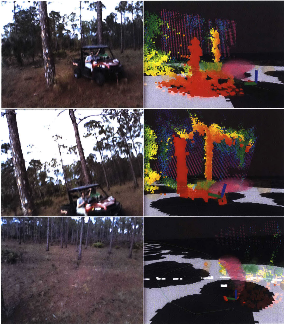
Figure 3-13: Return, 5 m/s from Flight i. Quadrotor approaches a pair of obstacles (top), not that although the initial velocity is to the right, the A* planner does not encode dynamic constraints and plans a path to the left. The quadrotor instead dynamically avoids the car to the right, passing the car (bottom) and returning to level flight (bottom).
