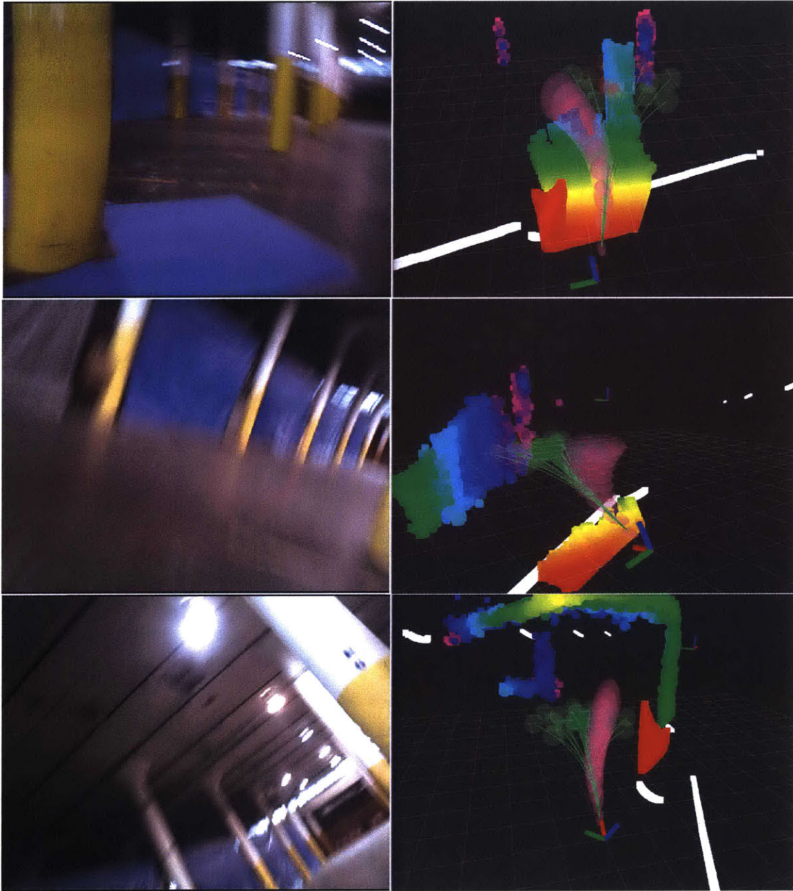
Figure 3-5: Outbound flight at 8 m/s. The vehicle approaches the first pillar and takes a different route than the previous flight, cutting sharply around the first pillar (top), quickly rolling and then choosing to come out of the turn (middle), aggressively coming out of this swerve at approximately 37\text{ deg} roll (bottom). Rotational motion blur in the RGB images is significantly higher than the 5 m/s flight.
