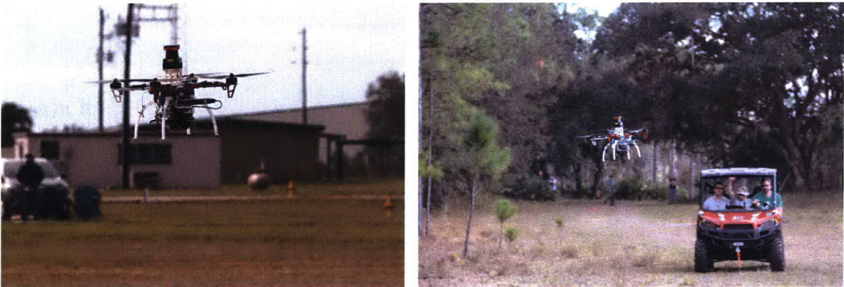
Figure 3-8: Draper-MIT quadrotor in configuration used for outdoor flight experiments, including with front-mounted Intel RealSense sensor and bottom-mounted Point Grey Flea3 camera. (Images courtesy of Jon How)
