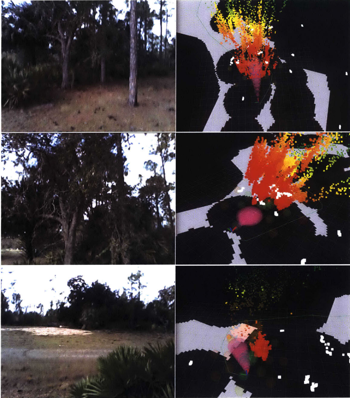
Figure 3-14: Demonstration of the global planner helping the vehicle get out of a dead end. The vehicle approaches a dead end (top) at 5\text{ m/s} (Flight i), chooses to stop to avoid collision (middle), and the global planner then guides the vehicle around to the left, out of the dead end (bottom).
