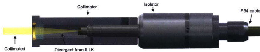
Figure 2-13: Diagram of a collimator produced by SPI Lasers to convert the diverging beam exiting their fiber laser fiber into a collimated beam [52].
