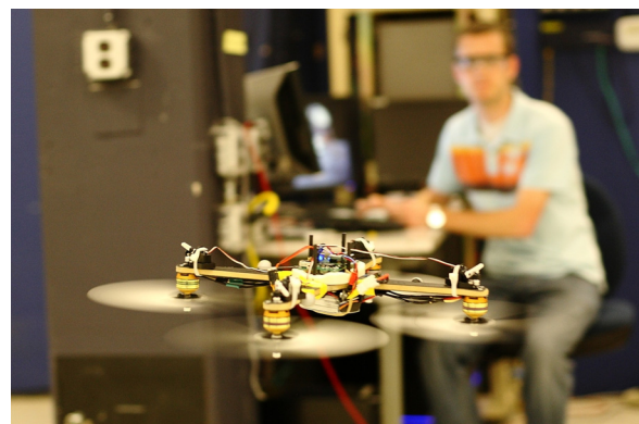
Fig. 1 The variable-pitch quadrotor during inverted flight. The symmetry introduced by the variable-pitch propellers allows the quadrotor to fly equally well upright or inverted.
