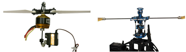
Fig. 13 Left: one of the pitch actuation mechanisms on the current version of the variable-pitch quadrotor. Right: a typical swashplate on a remote-controlled helicopter. (a) Variable-pitch actuator and (b) helicopter swashplate.
