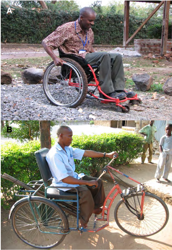
FIGURE 1. COMMONLY AVAILABLE MOBILITY AIDS IN DEVELOPING COUNTRIES. A) Conventional-style wheelchair. The user propels the wheelchair by grasping and pushing the pushrims attached to the wheels. B) Hand-powered tricycle. The user propels the tricycle via a hand crank system that drives either the front (shown) or rear wheels.
