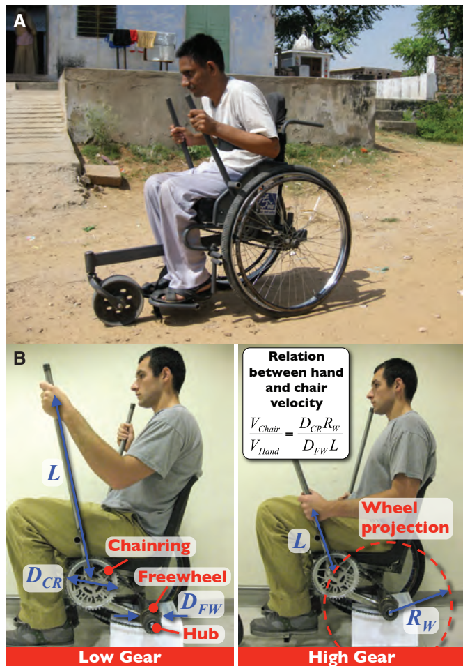
FIGURE 2. THE LEVERAGED FREEDOM CHAIR (LFC). A) An Indian trial subject using the LFC in his home village. B) LFC variable mechanical advantage, single speed drivetrain. All components in the drivetrain are made from single-speed bicycle parts found anywhere in the developing world. Inset gives the mathematical relationship for how the ratio between LFC speed ( V_{Chair} ) and pushing speed on the levers ( V_{Hand} ) varies as a function of the effective lever length ( L ), which is determined by hand position on the levers. Other labels: diameter of the chainring ( D_{CR} ), diameter of the freewheel ( D_{FW} ), and rear wheel radius ( R_W ).
