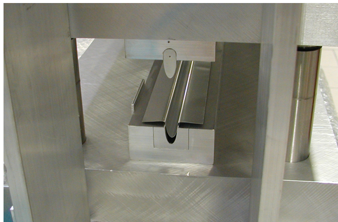
Figure 4: The target cell foil in the pneumatic press before (a) and after (b) shaping
