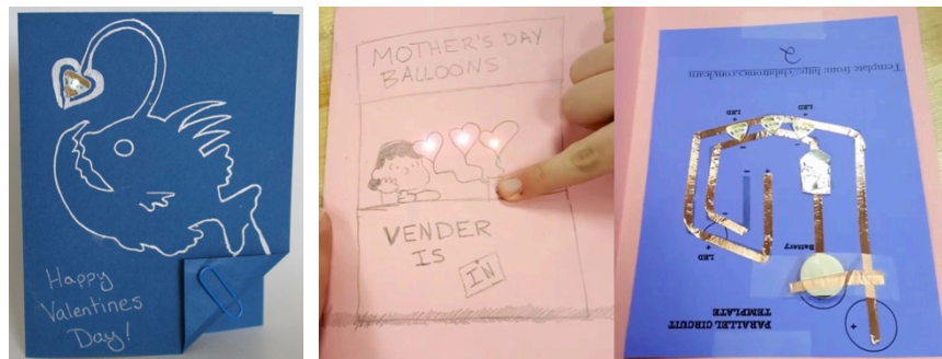
Figure 4.1. Light-up greeting cards made with paper circuitry. Valentine's Day card from Yukonstruct Makerspace (left) and Mother's Day card (center and right) from student of Colleen Graves. Circuit Sketchbook template is used to illuminate this card.
