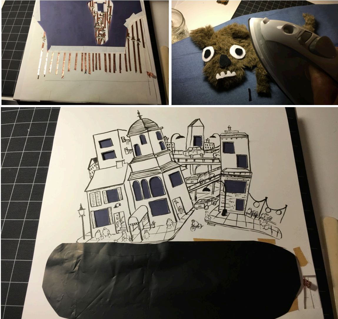
Figure A.10: TickyTown final construction process: vellum overlay (upper left), textile tog (upper right) and Velostat pressure sensor (bottom). Images by K-Fai Steele
