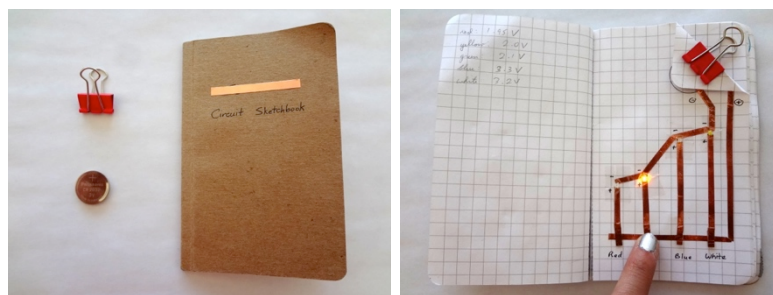
Figure 3.3. Standard sketchbook with coin cell and binder clip power supply. Example page.
