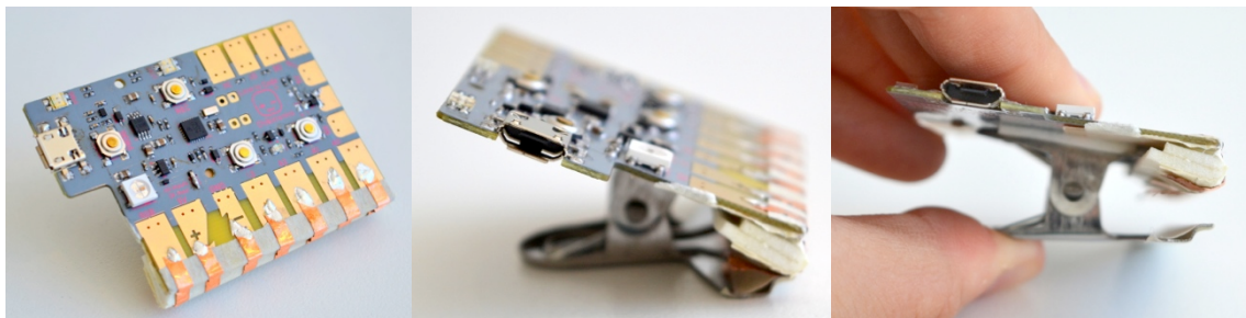
Figure 8.4: Code clip front view (left), side view (center) and open clip (right).
