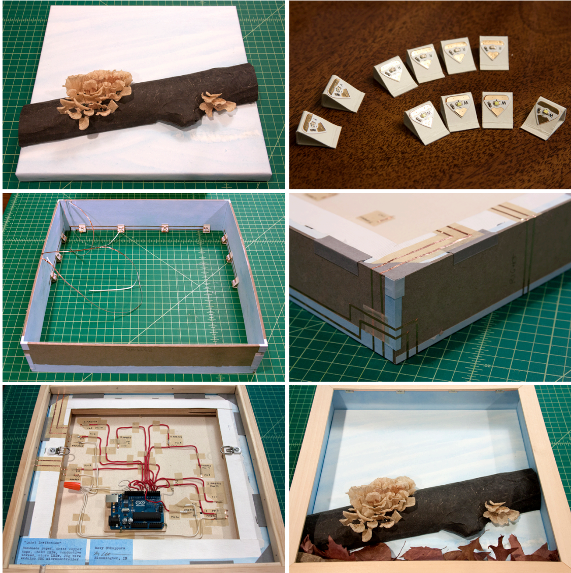
Figure A.25: From left to right, top to bottom: Assembled log circuit, frame LEDs, frame with assembled LEDs, circuitry wrapping around edge of canvas, circuitry controlled by Arduino and final circuitry assembly for Quiet Invitation by Mary Uthuppuru
