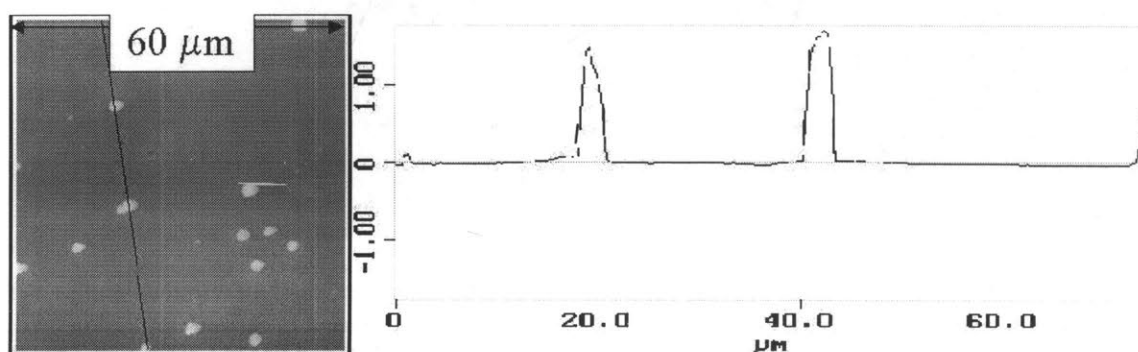
Figure 8.10. Representative AFM topography image and cross-section of embedded latex sphere surface. Cross-section y-axis is in μm.
