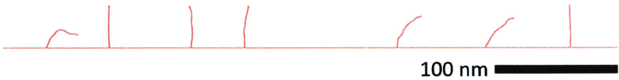
Figure 4-7: Partitioning can control ridge number and height. Pinning graphene to the substrate to eliminate sliding of graphene over substrate enables control of ridge number. Eliminating sliding effectively eliminates ridge-ridge annihilation and allows ridges to form on opposite sides of the pinned graphene.
