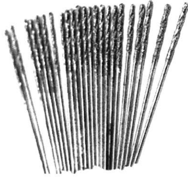
Figure 15 - Electroplated diamond twist drill bits for micro-drilling Vaca Muerta Shale.
