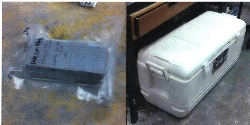
Figure 20 – Shale sealing and storage. Left: shale is stored in vacuum sealed bags to preserve in-situ water content. Right: cooler container for added protection. From Morgan (2015).
