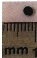
Figure 55 - O-ring seal which sits in the circular recess on the back side of the housing. When pressure is applied, the O-ring seals around the injection needle, preventing needle movement or leakage.
