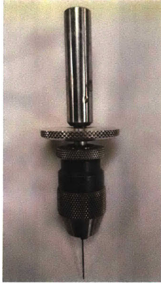
Figure 16 - Hand-feeding sensitive chuck adapter for micro-drilling.
