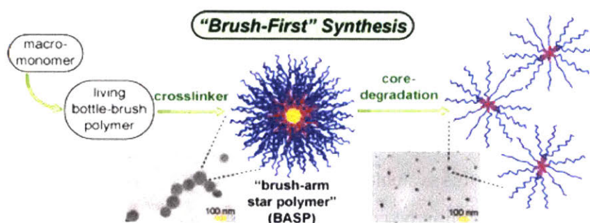
Figure 1.1: A brush-arm star polymer (BASP) can be synthesized using graft-through ROMP of macromonomer then crosslinker addition. Given the use of a photodegradable crosslinker, these BASPs can be degraded at the core with light irradiation to break the BASP into smaller components.
