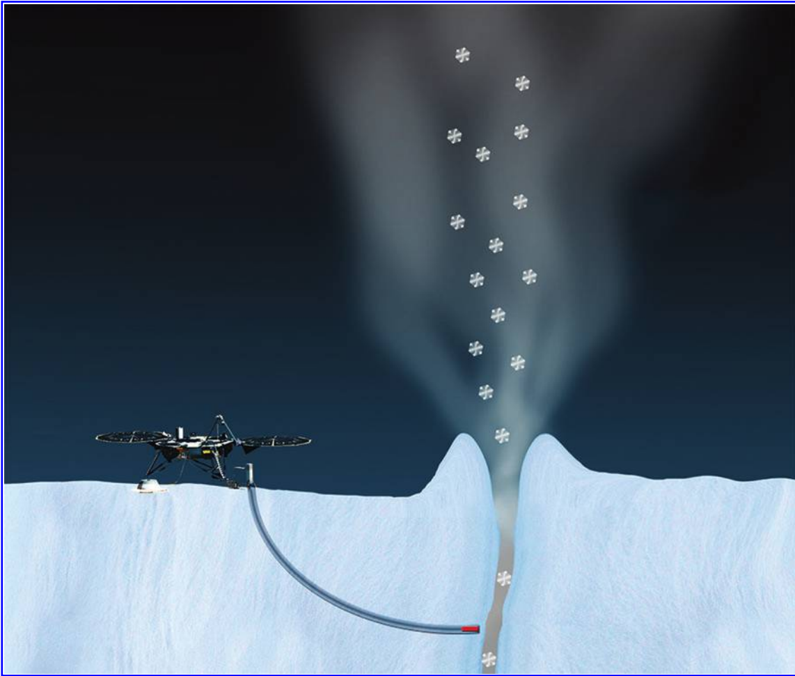
FIG. 7. Artist's concept of IceMole sampling strategy. The probe melts through the ice to encounter water near a plume, while the rover remains at a safe distance. [Concept: Enceladus Explorer (EnEx) consortium/German Space Agency (DLR)]
