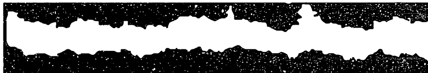
Figure 8.1 A magnified view of a single line ( 88.7 ). Grain size: 28\mu\text{m} . Measured diameter: 153 \mu\text{m} ; Std. Dev: 24 \mu\text{m} ; ( by occlusion )
