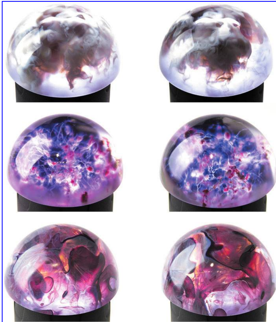
FIG. 4. A collection of three general examples of the data-driven material modeling approach, illustrating an array of internal material compositions achieved through the implementation of the described methods to achieve visually complex patterns. Such material compositions are uniquely obtained through our computational framework in combination with on-slice-time advection. The first row shows an example of advection driven by a given velocity field. The second row shows a volumetric data set where advection in the normal direction is used to create a diffusive effect in dense areas. The third row shows a periodic implicit function perturbed by a velocity field. For each set of 3D-printed objects, the two photographs depict the object from different viewing angles. All examples were produced on a Stratasys J750 full-color multimaterial 3D printer in collaboration with Stratasys Ltd. Photos: Mediated Matter.
