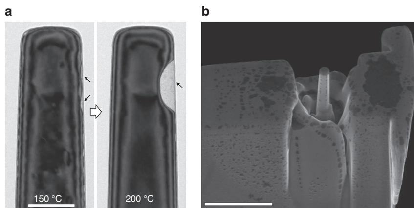
**Figure 4 | Distribution of giant cavities on sample surface.** (a) Formation of a giant cavity at the same location as the largest proto-cavities at the side of the pillar, as marked by the arrows. (b) SEM image viewed from 45° of a larger sample area after the same hydrogenation and heating treatments. Giant cavities not only formed at the top of the pillar, but also at the plane surface of the plate. Scale bar: (a) 200 nm, (b) 2 μm.
