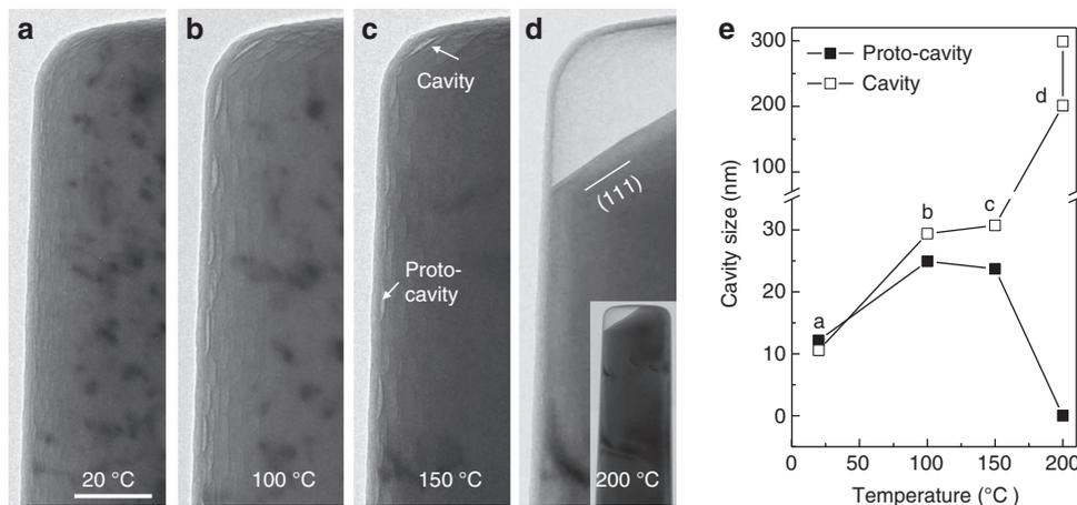
**Figure 3 | Formation of a typical giant cavity at  $\text{AlO}_x\text{-Al}$  interface.** See the Supplementary Movie for the dynamic process. (a–d) Snapshots of the pillar at 20, 100, 150 and 200 °C, respectively. (e) Size evolution of the proto-cavities and cavity with temperature. From 20 to 100 °C, the proto-cavities grow, but as the cavity on the corner begins to grow, the proto-cavities decrease in size. Scale bar, 100 nm.
