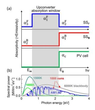
**Figure 2. Spectrally-selective surfaces**. (a) Step-wise absorption/emission characteristics of the spectrally-selective surfaces of the up-converter and the PV cell in Fig. 1. (b) The AM1.5D spectrum and the thermal radiation spectra at high temperatures. The approximation of the solar spectrum as the 6000K angularly-restricted blackbody spectrum is included for reference.
