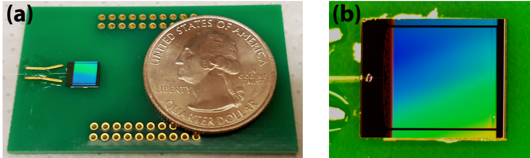
Figure 5-2: (a) Image of the silicon 4\times 4\text{ mm}^2 phased array next to a quarter. (b) Optical micrograph of the same phased array with epoxied input fiber.
